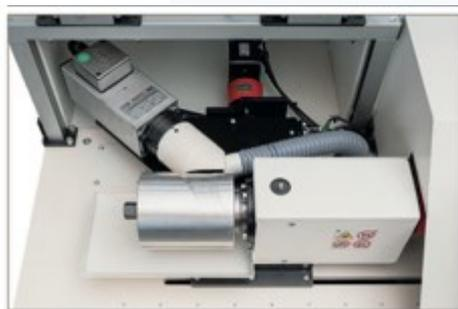
with skiving – using user-friendly 3D CAD software, which then automatically generates the mould machining program. The resulting mould dimensions are 120 mm in diameter and 180 mm in length. All machining settings can be modified and saved for future operations.
